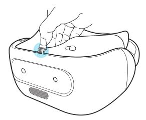
3. Insert the microSD card, with the gold contacts facing out, into the slot.
